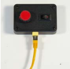
Manual speed control Can be used as a backup speed control instead of the DM-2A
