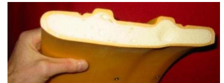
Strong - "Space Age" lightweight but stiff foam sandwich construction.
